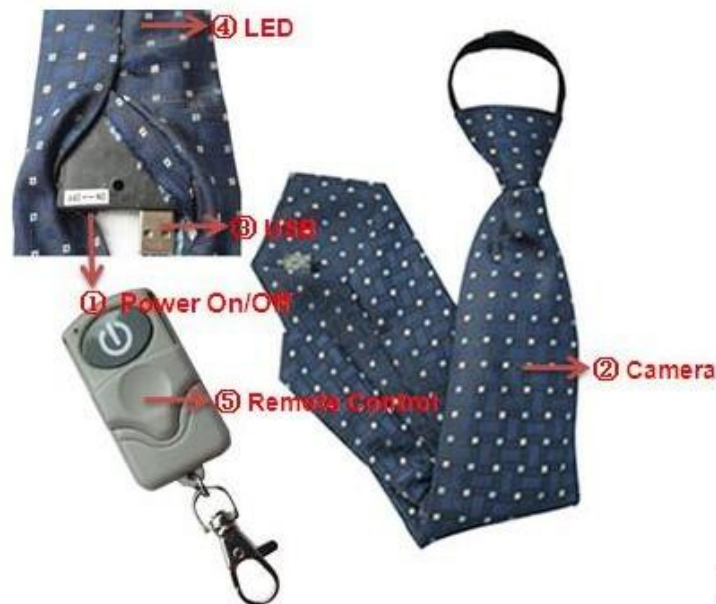
1. Power on/off 2. Camera 3. USB Port 4. LED 5. Remote Control
